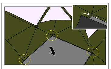
Add the flooring provided to help contain the heat in the sauna. All 4 edges of the flooring is attached by velcro at all 4 corners of the tent skirt. This step is optional and if flooring is used be careful with the ashes from the furnace because it will burn a hole through the flooring fabric.
